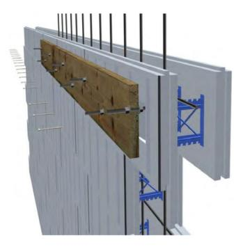
**Step 5:** Place and consolidate the concrete into the forms. Use pencil vibrators, target mix, and super plasticizers to ensure good flow and consolidation around the anchors, and into the cut-outs.
