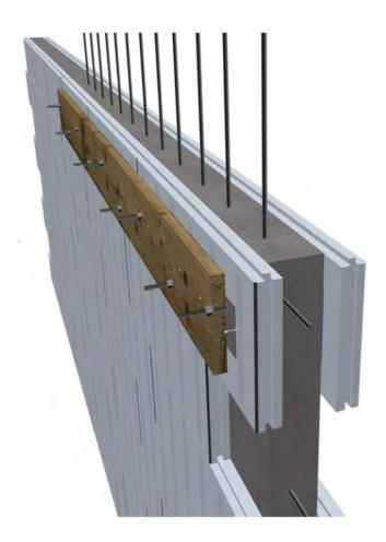
**Step 6:** After suitable cure time, continue with the installation of joist hangers and complete joist construction.
