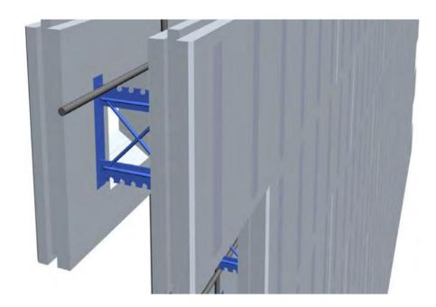
**Step 2:** Place horizontal and vertical reinforcing steel as per manufacturer's or engineer's specifications.
