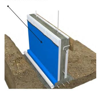
**Step 7:** If coarse, clean granular material, or a drainage mat are applied adjacent to the foundation wall, it must extend to the footing drain level to facilitate drainage to the footing drain.
