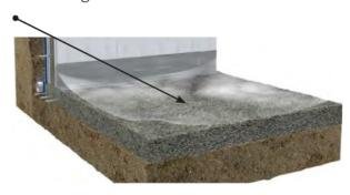
**Step 11:** Apply compatible, flexible sealants at the slab/wall transition and around all penetrations through the slab as part of the required air barrier and soil gas control in regions where soil gas is known to constitute a hazard, and as a requirement of slab airtightness.
