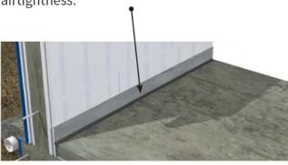
**Step 9:** Place not less than 100 mm of coarse clean granular material under the slab-ongrade. This layer provides a capillary break for ground water and controls liquid water being drawn up to the slab above and resultant moisture damage to floor finishes. This is required where soil gas provisions are required, and is otherwise considered best practice.
