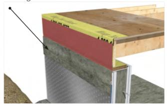
**Step 20:** Frame and tilt wall into place. Turn the SSM flap upward and staple it in place.
