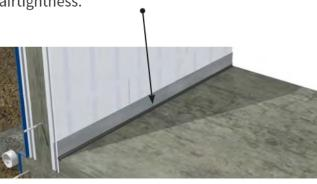
**Step 8:** Place not less than 100 mm of coarse clean granular material under the slab-ongrade. This layer provides a capillary break for ground water and controls liquid water being drawn up to the slab above and resultant moisture damage to floor finishes. This is required where soil gas provisions are required, and is otherwise considered best practice.
