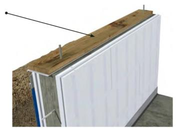
**Step 13:** Drape a strip of synthetic sheathing membrane (SSM) over the plate. Carefully perforate the SSM to allow the anchor bolts through.
