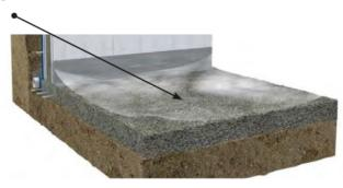
**Step 10:** Apply compatible, flexible sealants at the slab/wall transition and around all penetrations through the slab as part of the required air barrier, and soil gas control in regions where soil gas is known to constitute a hazard, and as a requirement of slab airtightness.
