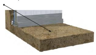
**Step 9:** Install polyethylene or type S roll roofing under the slab-on-grade as required dampproofing and also to serve as part of the soil gas control measures for areas where soil gas is known to constitute a hazard.
