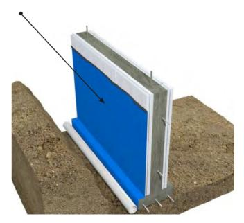
**Step 6:** If coarse, clean granular material, or a drainage mat are applied adjacent to the foundation wall, it must extend to the footing drain level to facilitate drainage to the footing drain.
