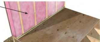
**Step 23:** Complete the installation of the drywall and interior finishes. Insulate the rim joist region using extruded (EPS) or expanded polystyrene (XPS) foam insulation. Low expansion air sealing foam can be used to achieve continuity of the air barrier through the rim joist. Other methods of insulating the rim joist could also be used.
