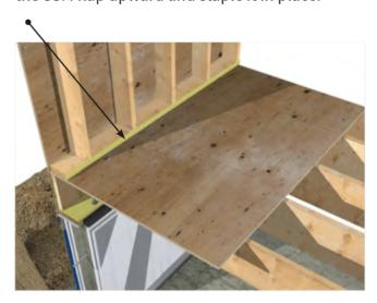
**Step 17:** Apply SSM tape to seam for airtightness.
