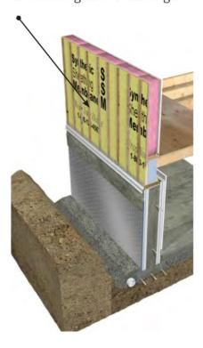
Step 26: Install the selected cladding using corrosion-resistant fasteners. Back fill the excavation and complete all landscaping with a slope away from the foundation.
