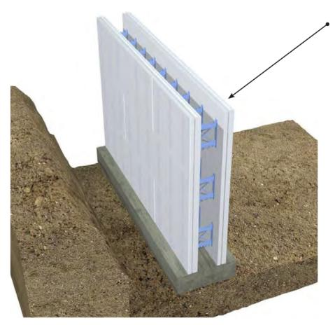
Step 3: Install the ICF system forms onto the footing. Integrate the horizontal steel progressively as the forms are placed and tie any horizontal steel to the form webs as necessary to ensure proper alignment during concrete placing.
