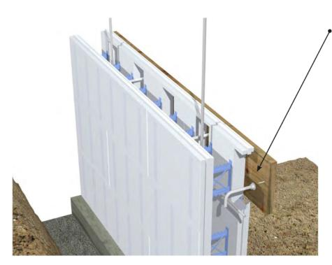
**Step 4:** The floor structure can be supported by joist hangers attached to a ledger fastened to the interior of the wall as shown as shown in this section. The ledger must be at least 38 mm thick and the depth of the supported floor joists, and must be fastened to the ICF foundation with anchor bolts in accordance with Part 9 of the code. Alternately, the floor structure can be installed onto a plate at the top of the ICF foundation wall as shown in 3.1.06b.
