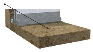
**Step 10:** Install polyethylene or type S roll roofing under the slab-on-grade as required dampproofing and also to serve as part of the required soil gas control measures for areas where soil gas is known to constitute a hazard.
