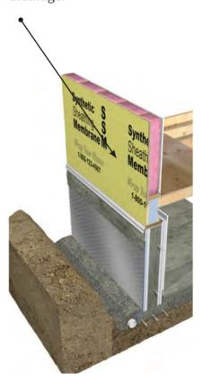
**Step 25:** If desired, or required by cladding manufacturer, install treated wood strapping to the wall and insect screen at regions terminating above flashings.
