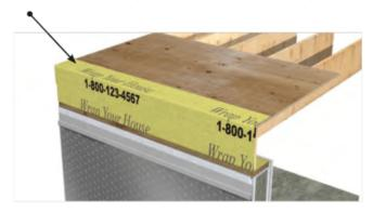
**Step 18:** Parge or protect the surface of the ICF from six inches below grade up to the sill flashing.
