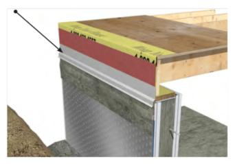
**Step 21:** Install selected insulation in the wall cavities, and apply acoustic sealant to the flap over the bottom wall plate.
