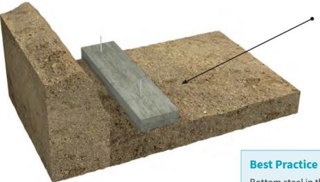
**Step 2:** Cast the footing to the required dimension with approved concrete. The ICF foundation wall is required to be formed on a footing with a shear key, or with 15 m vertical steel reinforcing dowels at a minimum 1.2 m o.c. (shown).
