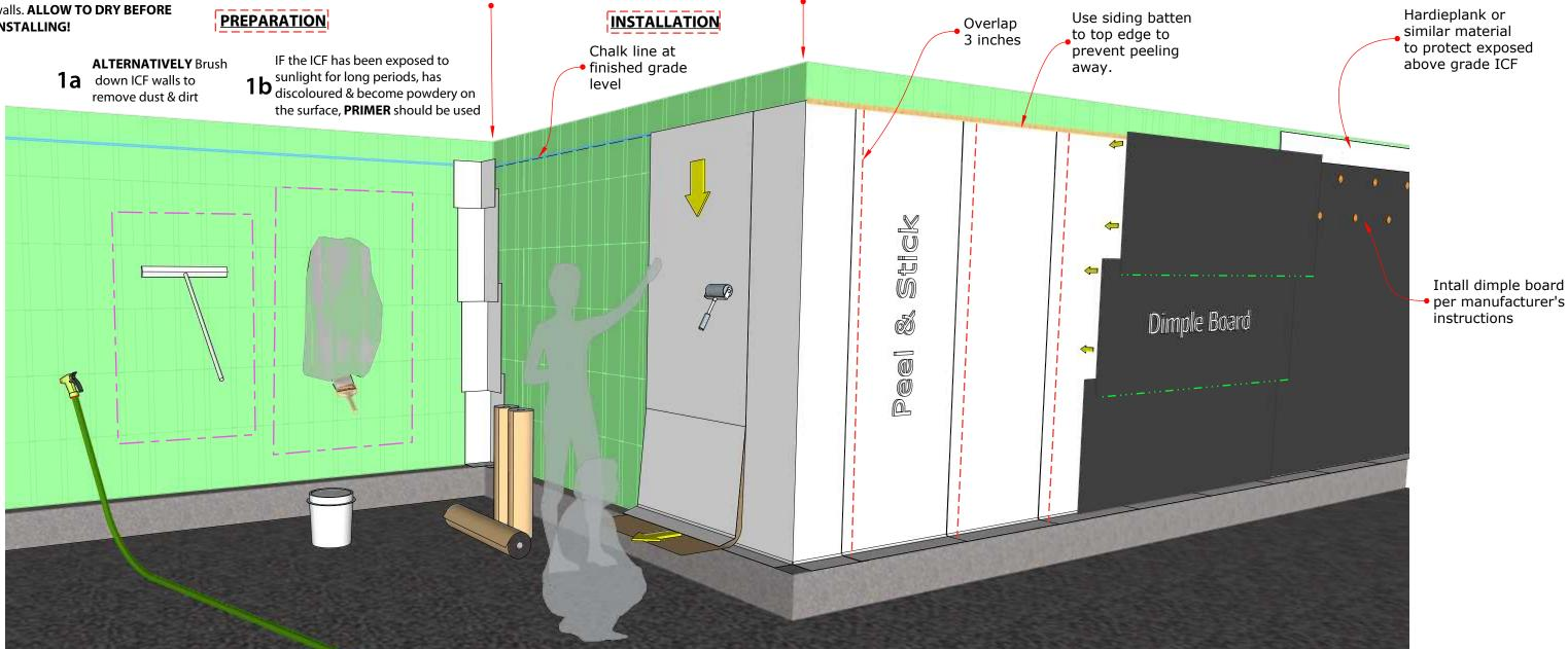
PEEL & STICK: Self-adhesive waterproofing membrane specifically for application to ICF.
